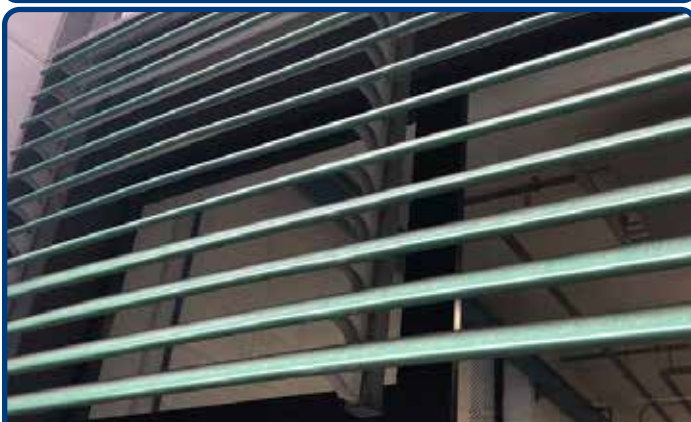
SUN LOUVRES SOLAR SCREEN LINEAR PANELS 84R Linear stripes 84R windproof width mm.84 rounded edges clip-on main supporting stringers inclination 30° - 45° - 65°-22°. Pre painted aluminium for external use 100% humidity resistant corrosion proof saltiness Incombustible Euroclass A1
