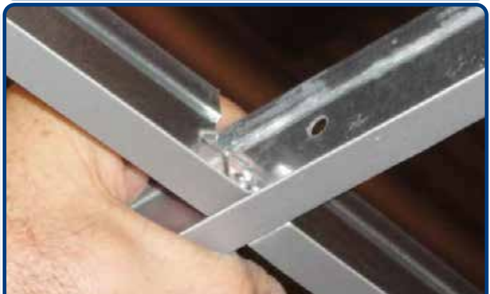
EXPOSED T SUSPENSION GRID FOR LAY-IN CEILING TWIN LOCK reticular grid T section mm.24 height mm.38 main runner and cross tees mm.600-1200 made of hot dipped galvanized steel with exposed pre painted aluminium capping washable 100% humidity resistant corrosion proof saltiness Incombustible Euroclass A1
