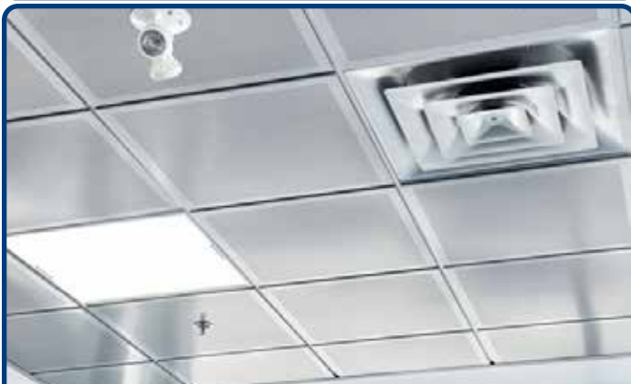
PANELS False ceiling panels mm.600x600 concealed systems CLIP-IN and LAY-IN LAY-ON T 24-15 exposed suspension grid system. Pre painted aluminium and steel Incombustible Euroclass A1
