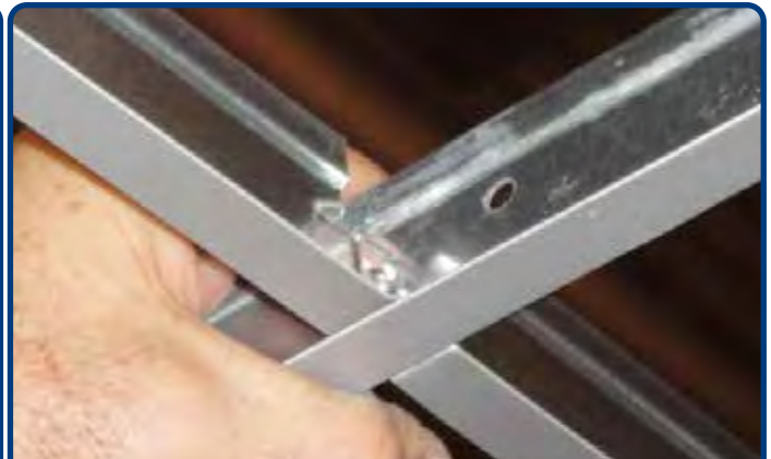
EXPOSED T SUSPENSION GRID FOR LAY-IN CEILINGS TWIN LOCK reticular grid T section mm.24 height mm.38 main runner and cross tees mm.600-1200 made of hot dipped galvanized steel with exposed pre painted aluminium capping washable 100% humidity resistant corrosion proof saltiness Incombustible Euroclass A1
